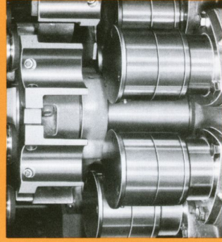
Six-station rotary seaming turret. Cans spinning during the seaming operation to permit close center spacing.
