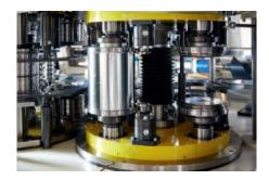
The latest development is the new series of CF 4xx, Perfectly designed to combine a wide working range of up to 200 mm diameter, quick change-overs of height and diameter and a remarkable production speed of up to 300 cpm.
